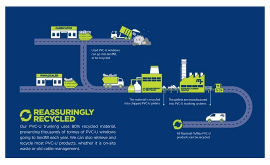
Marshall-Tufflex use 'post-industrial waste' windows (waste windows from window fabricators) or 'post-consumer waste' windows (windows that have come out of buildings at the end of their useful life). Because windows are designed to withstand external elements, they obtain a raw material that is more robust and higher quality than virgin PVC.
